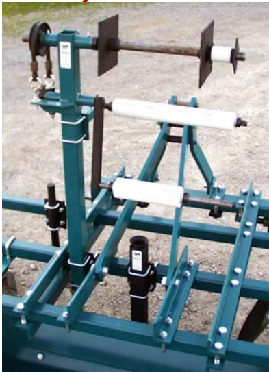
Right-hand tape layer installation with tape row in center
