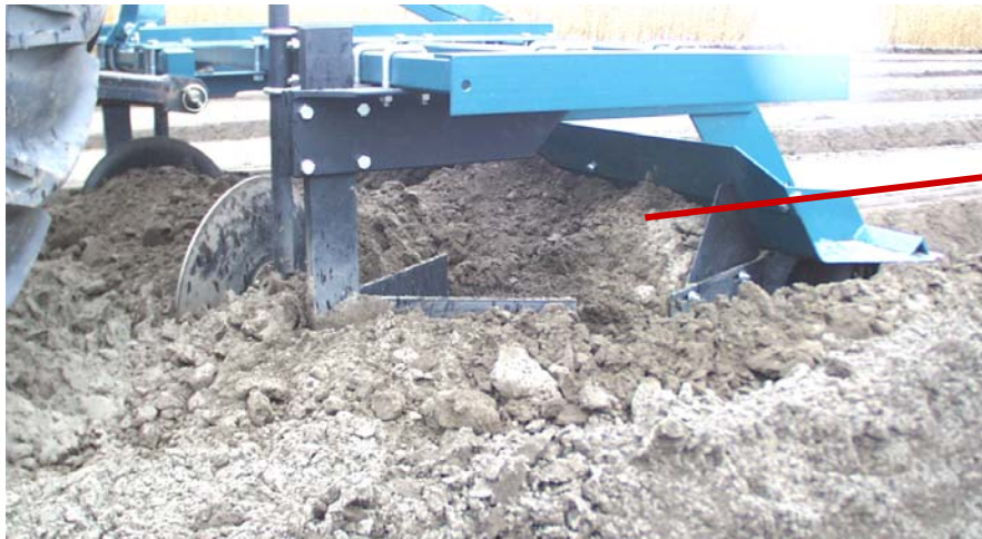
Photo is lightened to show typical soil build-up in front of pan
